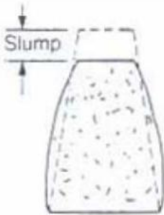
True Valid slump measurement 0-175 mm
